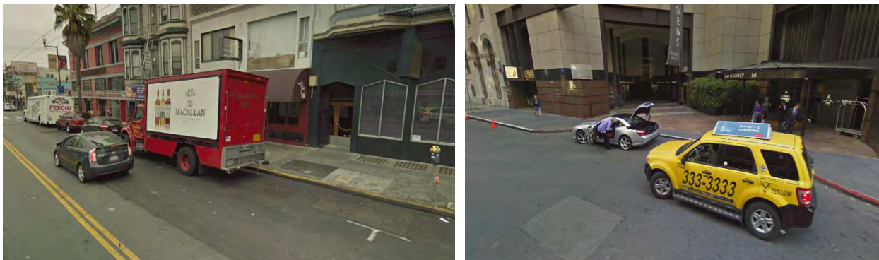
Figure 55: Two typical on-street loading facilities. Left: yellow curb (freight loading); right: white curb (passenger loading). Source: Google Street View, 2018.
