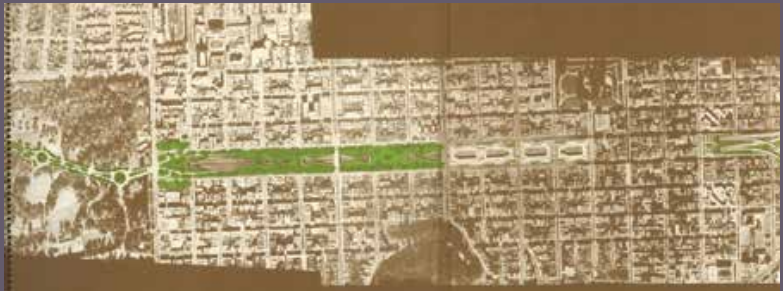
A 1966 design proposal for the un-built Panhandle Freeway intended to ameliorate the concerns of anti-freeway activists by placing the freeway partially underground.
