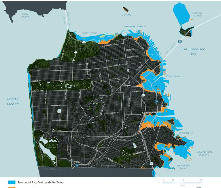
Figure 2.3 Comparison of the SLR Vulnerability Zone and H++ with 100-year Storm Surge
