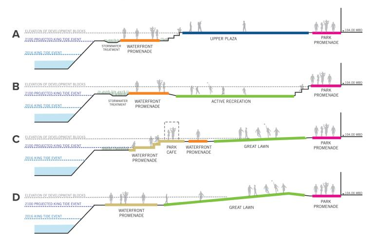
This diagram illustrates the relationship of Mission Rock program areas to each other and to key sea level rise (SLR) elevations. The finish grade elevations will be based on 2100 king tide elevations (SLR + storm surge).
