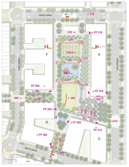
Figure 6.11-4: *Grading Diagram*
