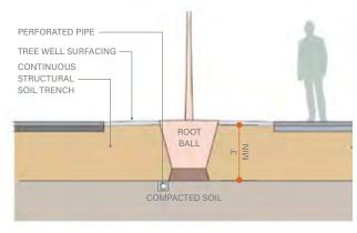
Figure 5.5–2: Typical Section of Sand-Based Structural Soil
