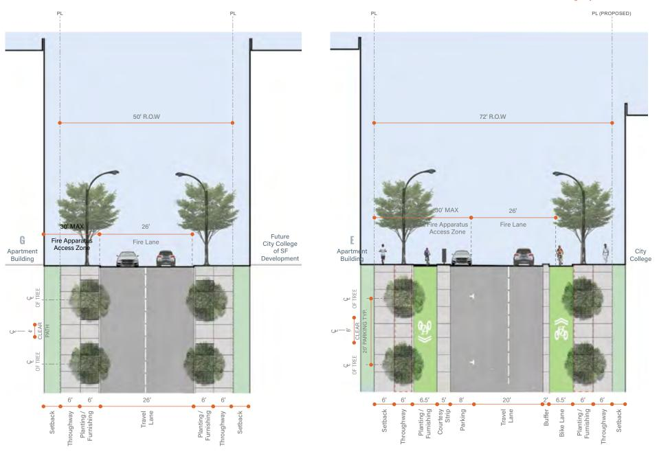
Figure 5.12–3: Lee Avenue, Section 1 \*see "Figure 5.12–2: Lee Avenue, Plan Enlargements L.1-L.5", Site Plan L.1
