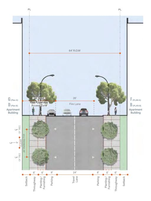
Figure 5.13-2: North & South Street, Section 1 \*see "Figure 5.13-3: North & South Street, Plan Enlargements N.1 & S.1
