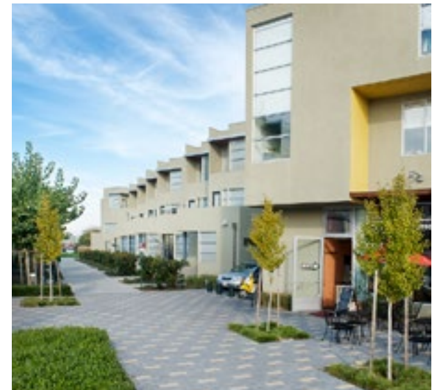
Fire access lane serves as pedestrian pathway
