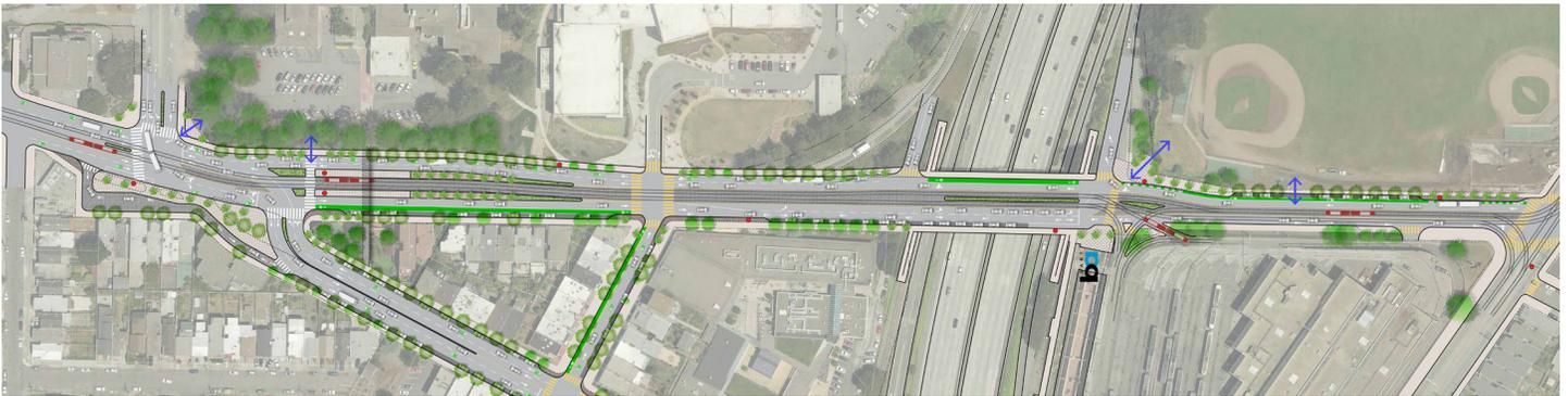
**2. The proposed design includes reconfiguring the Ocean/Phelan/Geneva intersection and creating a local access lane onto Geneva. This would maintain access for the properties on Ocean Ave, provide safer pedestrian crossings and create a public gathering place. This would involve additional study. What do you think of this idea? (Check  one)**
