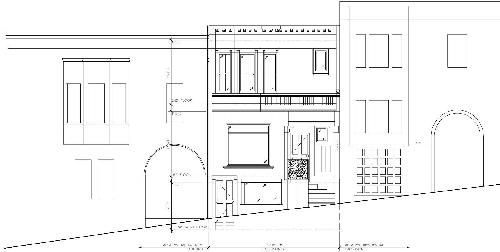
1 EXISTING EAST(FRONT) ELEVATION Scale: 1/4" = 1'-0"
