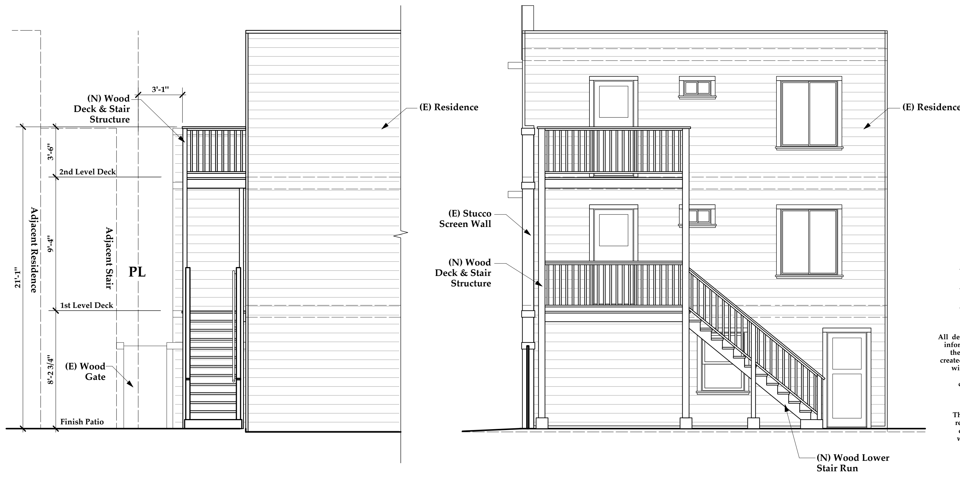
Partial North Elevation W/ (N) Deck & Stairs
