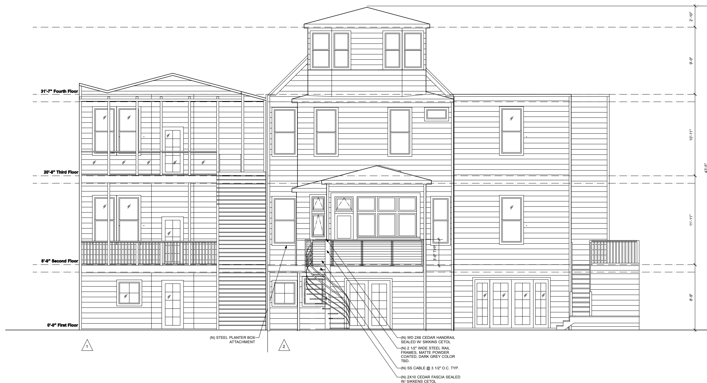
PROPOSED SOUTH ELEVATION Scale: 1/4" = 1'-0"
