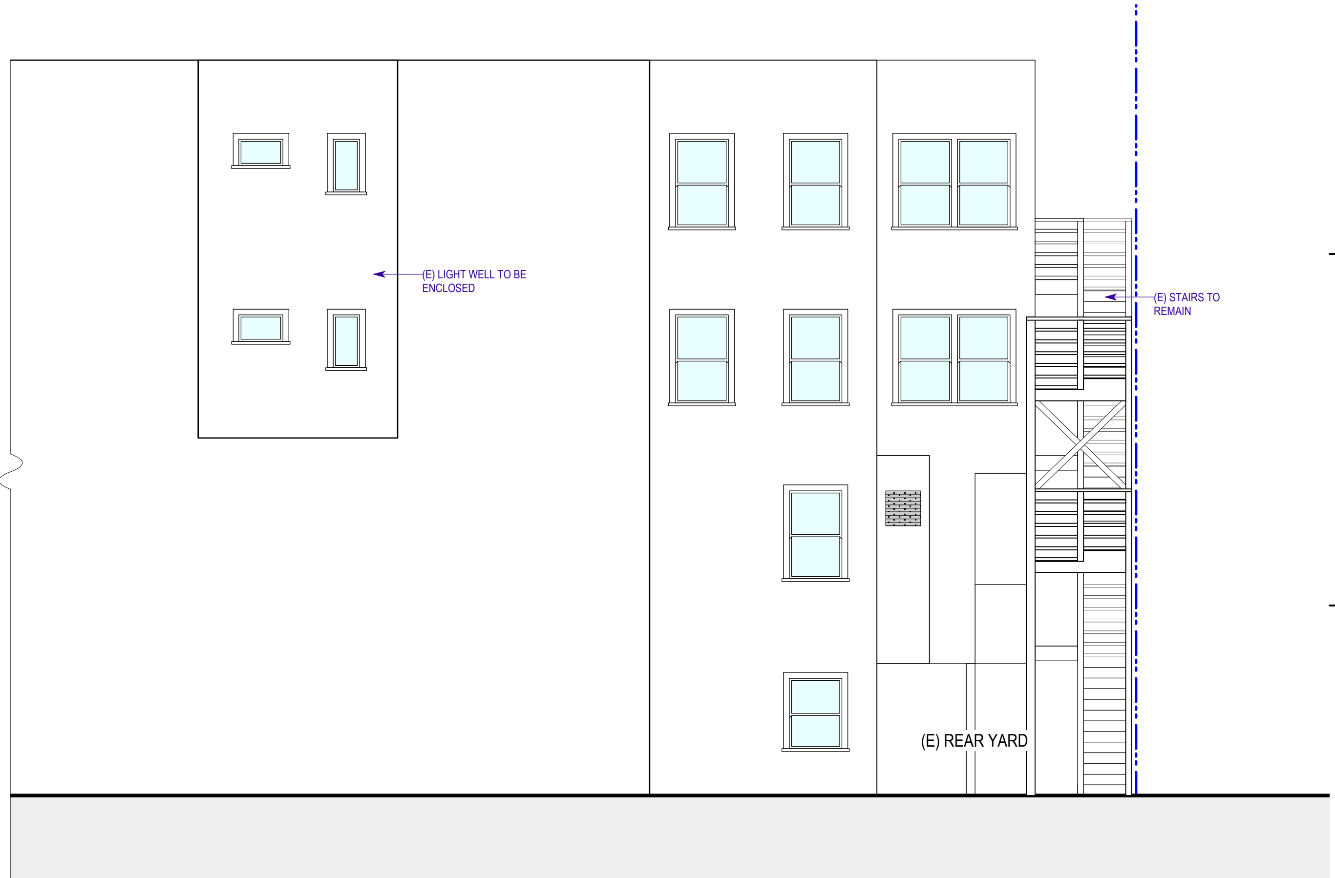
Existing Right Elevation 3/16" = 1'-0"
