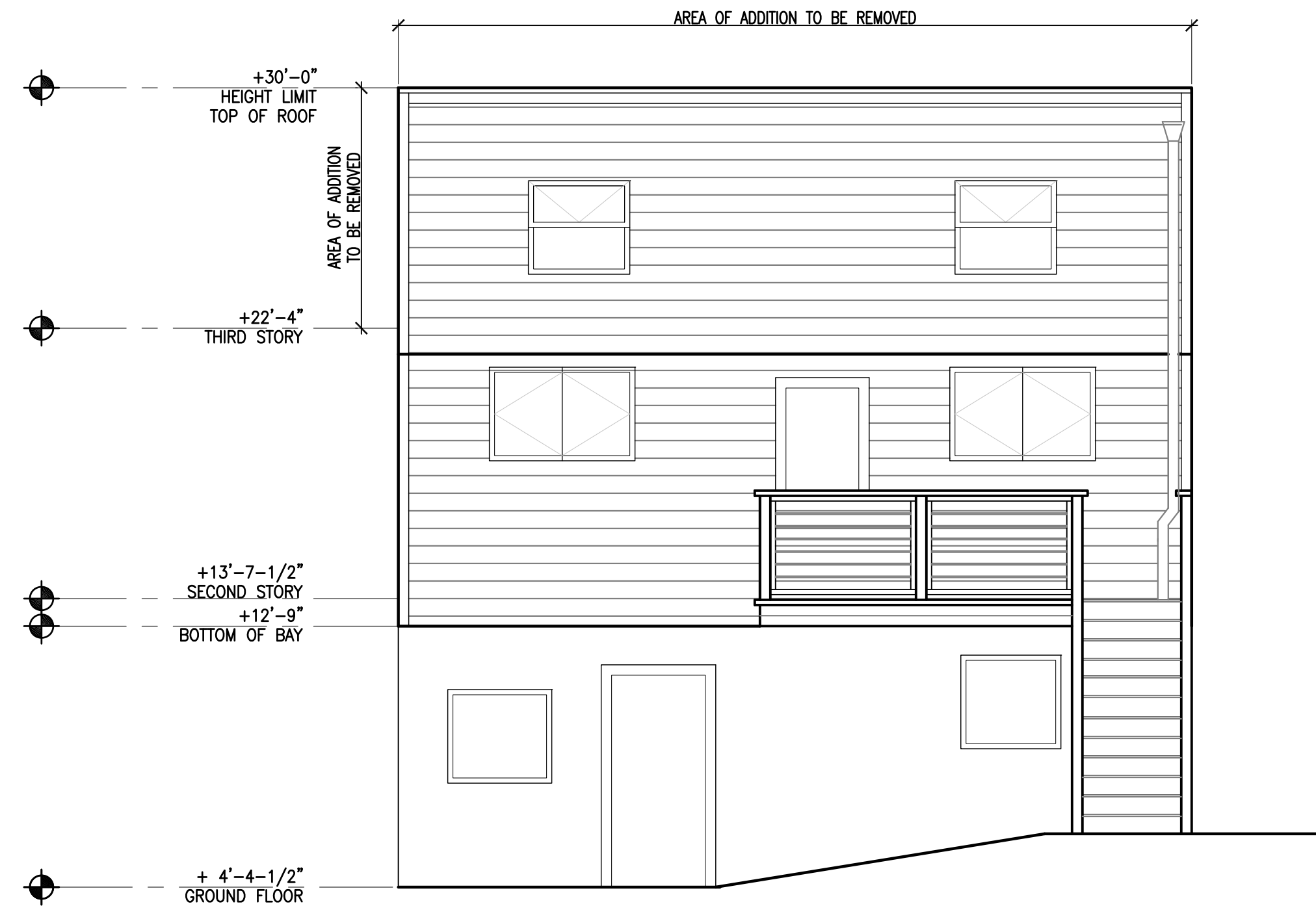
2 EXISTING SOUTH ELEVATION - REAR BUILDING A2.02 1/4" = 1'-0"
