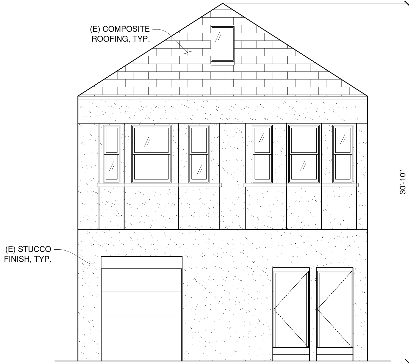
EXISTING FRONT ELEVATION SCALE: 1/4"=1'-0" (MAIN HOUSE)
