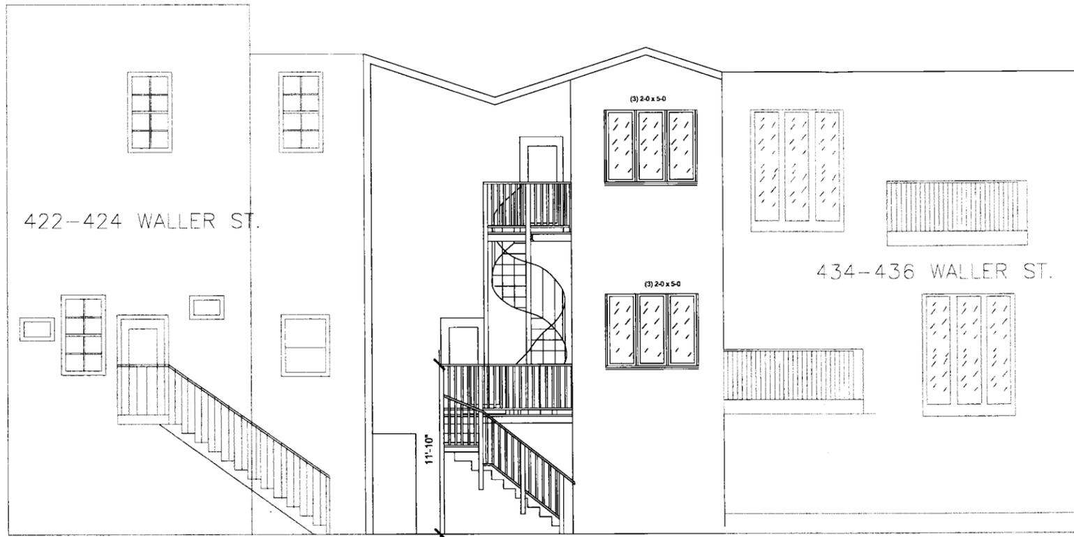
MATERIALS NOTE. THE NEW DECK RAILS AND STAIRS WILL BE MADE OF DECAY RESISTANT WOOD. THE WALLS AT THE FIRST FLOOR WILL BE FINISHED AND PAINTED TO MATCH THE EXISTING HOUSE. THE SPIRAL STAIRS WILL BE MADE OF STEEL WITH A BAKED EPOXY FINISH.
