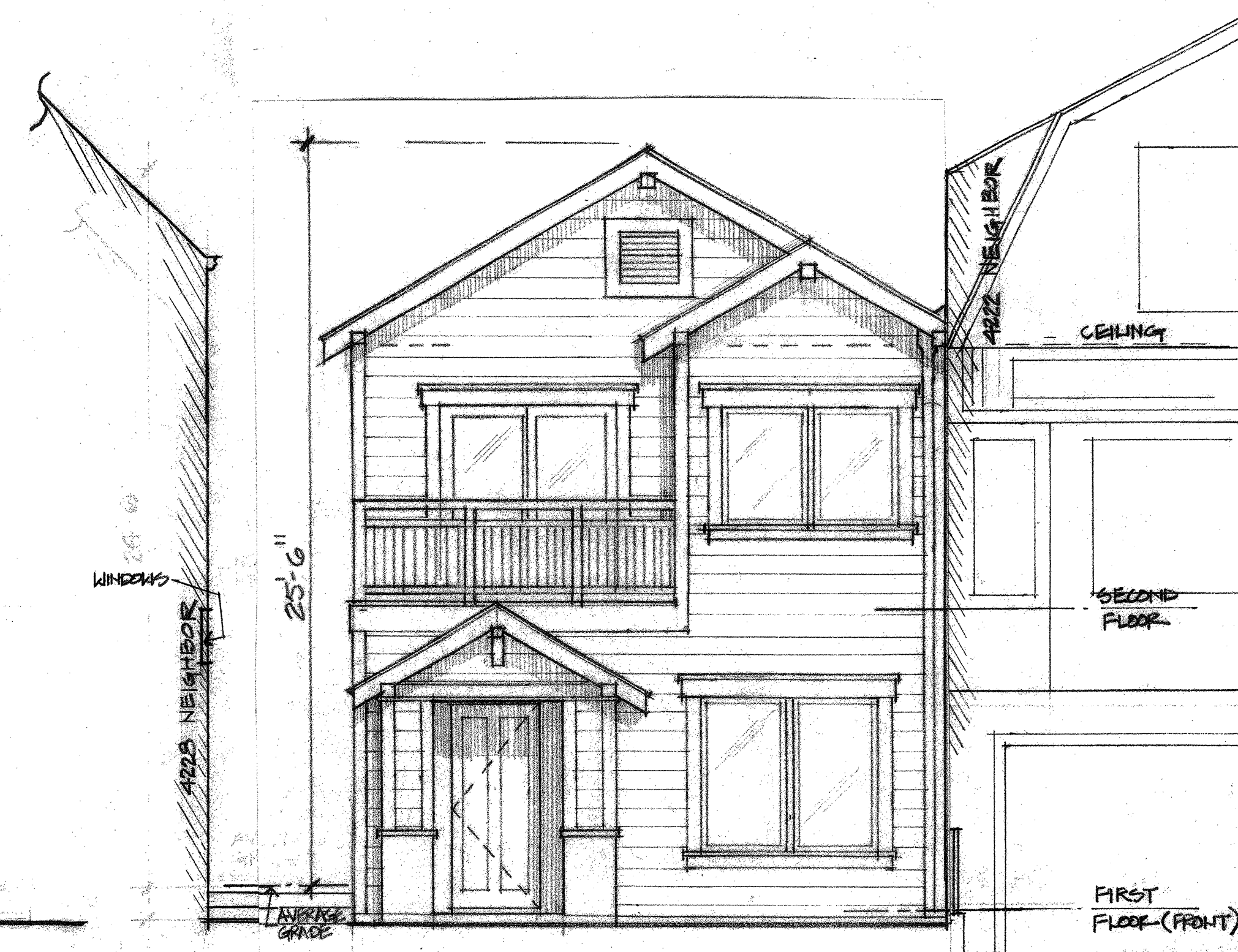
NEW SOUTH ELEVATION (FRONT) SCALE: \frac{1}{4}" = 1'-0"
