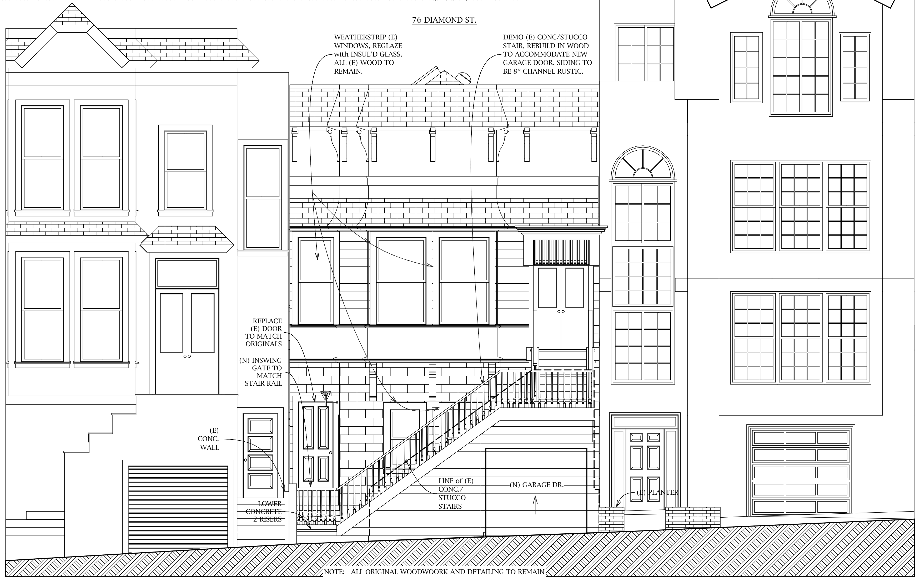
2 East (Front) Elevation SCALE: 1/4" = 1'-0"
