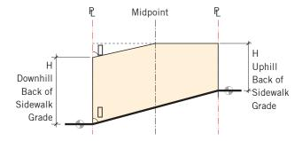
Figure 6.2.2 Measuring Height on a Slope
