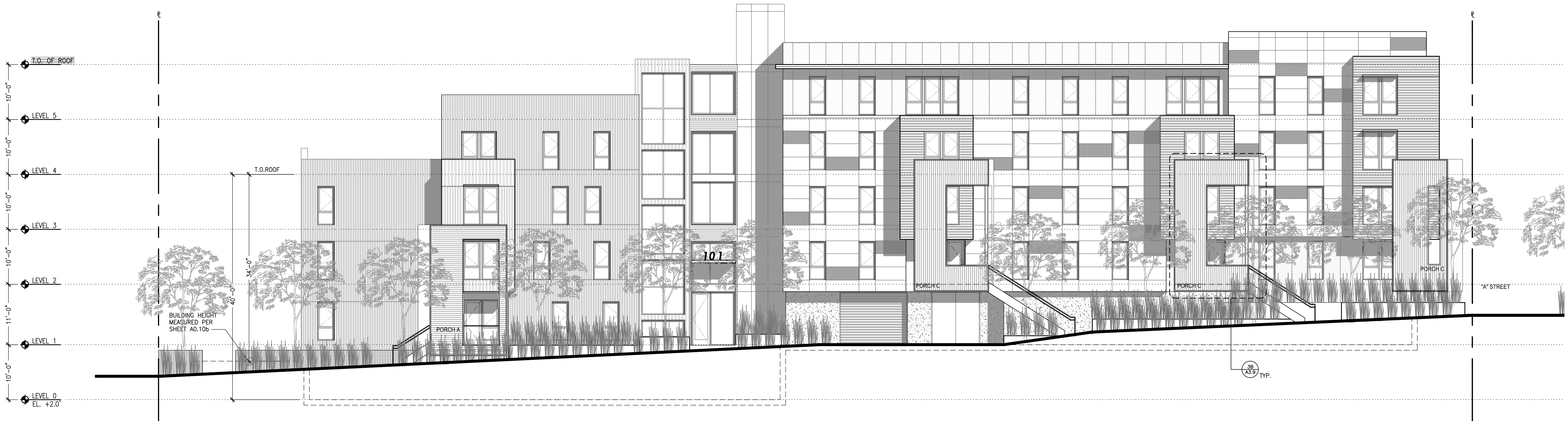
2 ELEVATION - CENTER STREET (NORTH ELEVATION) 1/8" = 1'-0"
