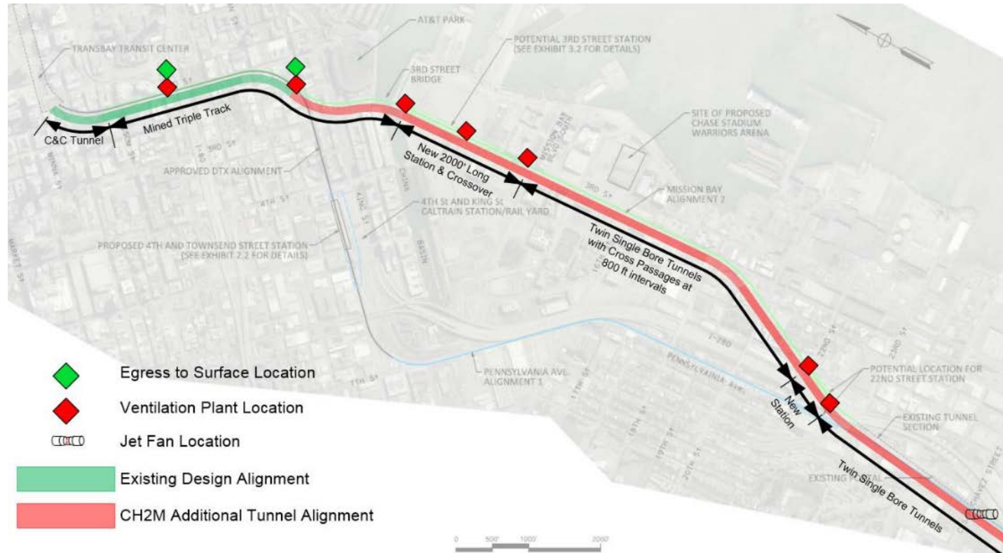
Figure 8: Mission Bay Alignment, Station Alternative 2 Ventilation Plan
