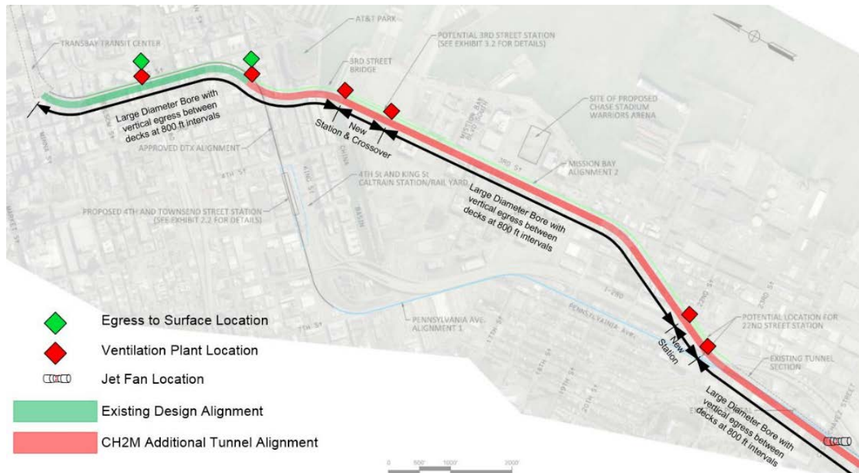
Figure 10: Mission Bay Alignment, Alternative 3 Ventilation Plan
