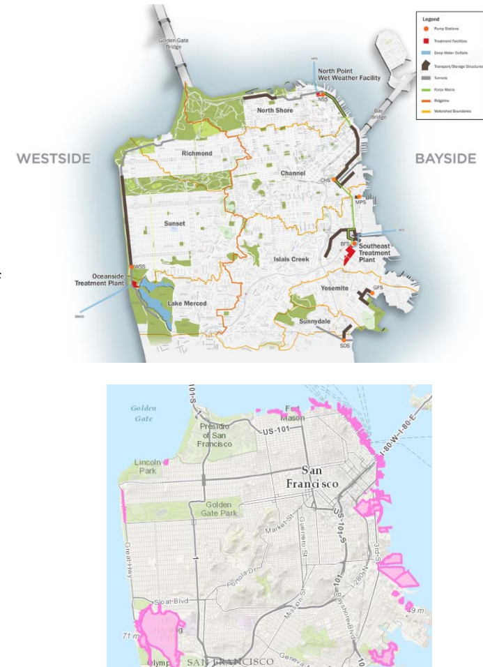
Figure 2 – San Francisco Stormwater Management Infrastructure. Top – Sewer System Improvement Plan shows major outlets and treatment facilities. Bottom – Municipal Separated Storm and Sanitary (MS4) Sewer Zones are shown in pink. Source: SFPUC
