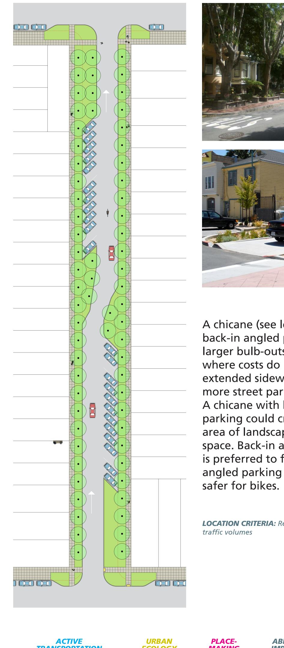
A chicane (see left) can include back-in angled parking and larger bulb-outs in instances where costs do not allow for extended sidewalks, or where more street parking is desired. A chicane with back-in angled parking could create expanded area of landscaping and public space. Back-in angled parking is preferred to front-loaded angled parking because it is
