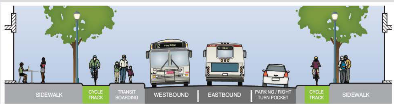
Folsom Street: typical section of proposed two-way scenario showing wider, well-furnished sidewalks, cycle tracks, and two-way transit service.
