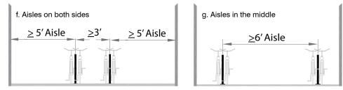
In cases shown in illustration (g) racks must be at least three feet from the wall to allow two bikes parked to one rack. If this distance is lower than three feet, such rack would only count for one bicycle parking space.
