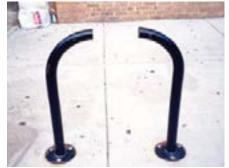
**Unacceptable** These bicycle racks either provide only one point of support for bicycles, are constructed with round tubed material which makes them prone to cutting, or do not allow locking a frame and wheel directly to the rack with a U-lock.
