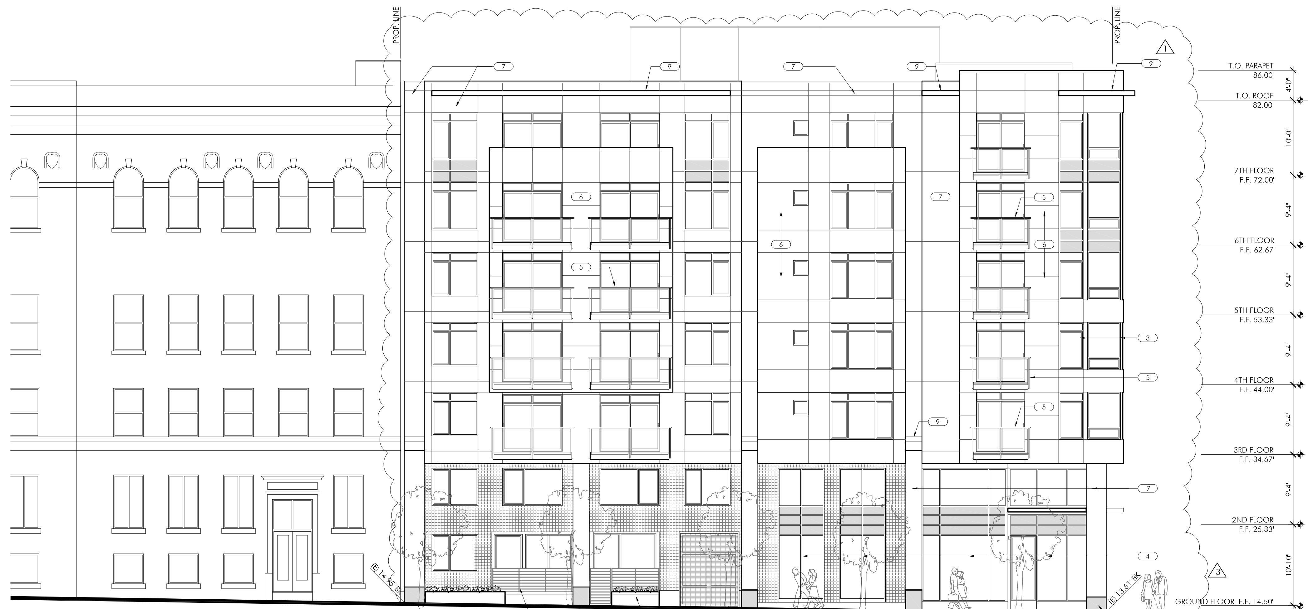
1 SOUTH EXTERIOR ELEVATION - 16TH ST. 1/8" = 1'-0"
