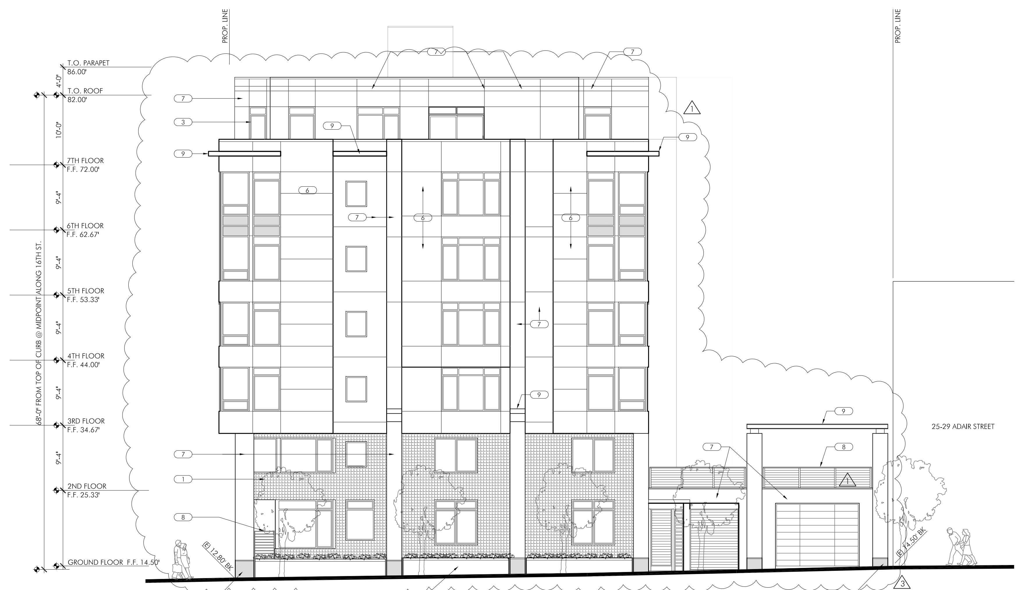
1 NORTH EXTERIOR ELEVATION - ADAIR ST. 1/8" = 1'-0"
