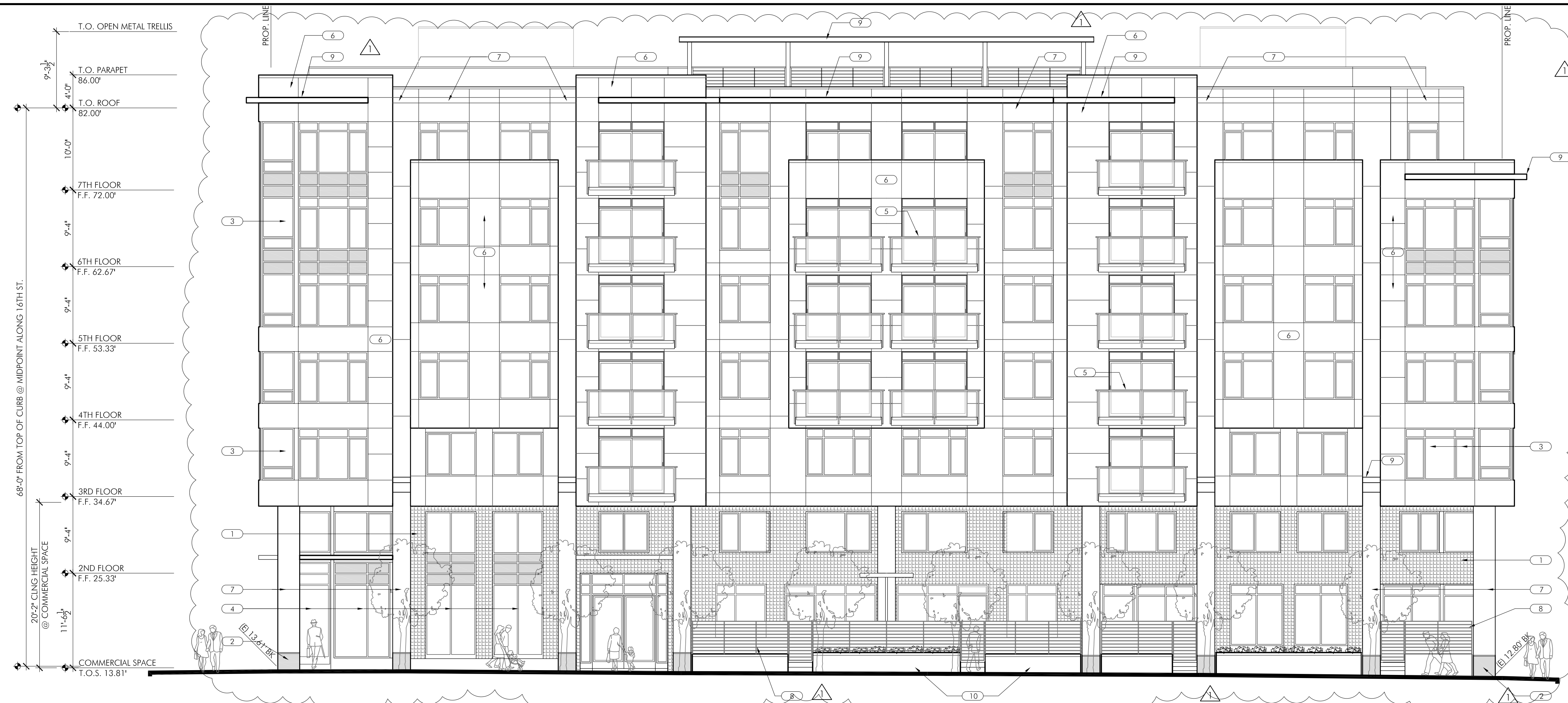
2 EAST EXTERIOR ELEVATION - S. VAN NESS AVE. 1/8" = 1'-0"
