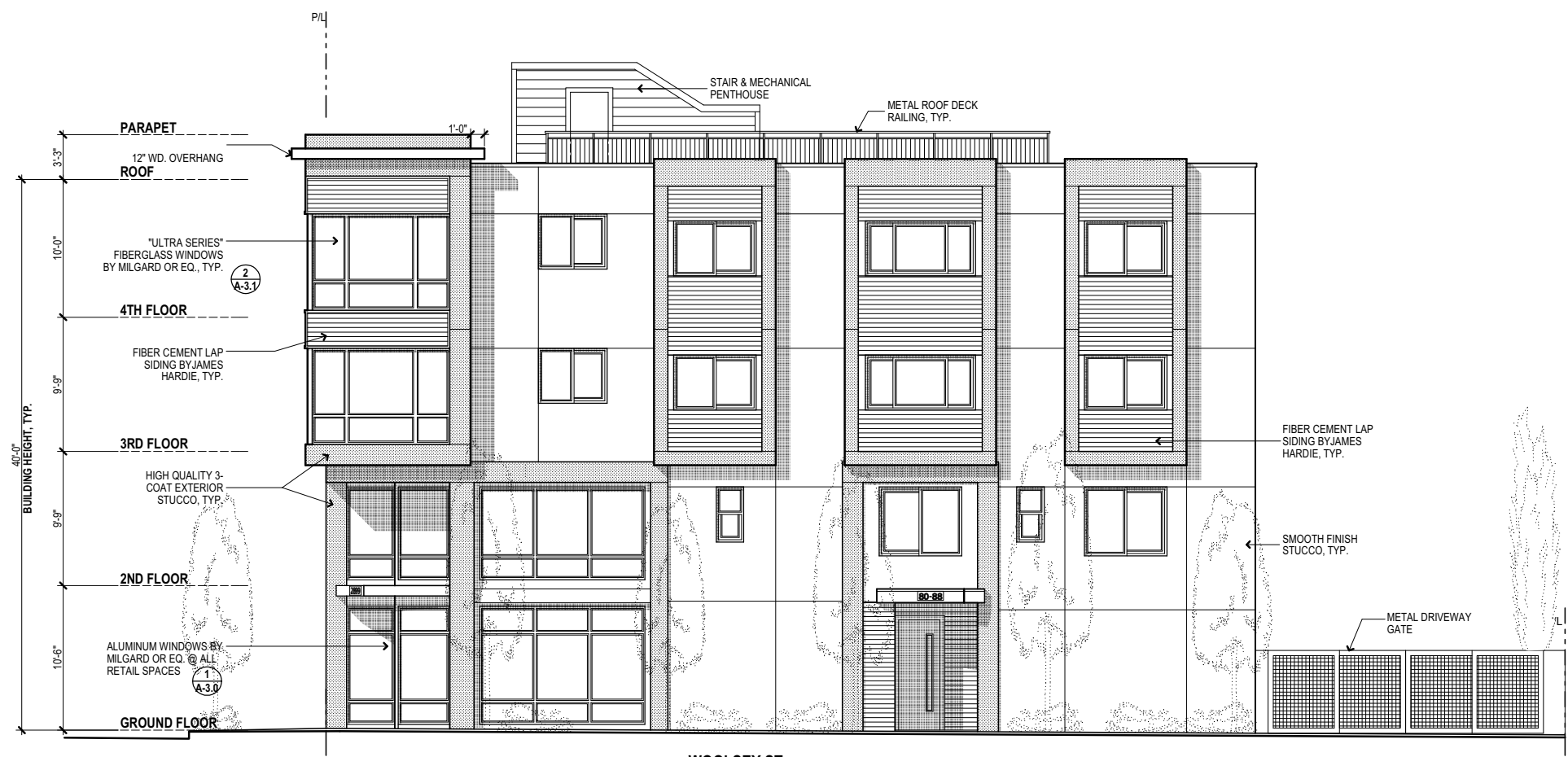
RIGHT ELEVATION WOOLSEY ST. ALL DIMENSIONS FROM FINISH TO FINISH, U.O.N. SCALE: 3/16" = 1'-0"
