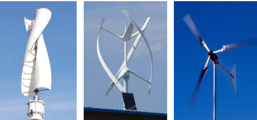
LEFT AND CENTER: Vertical axis wind generators may vary in appearance. Blades that present a solid appearance (such as the left image) are encouraged.
