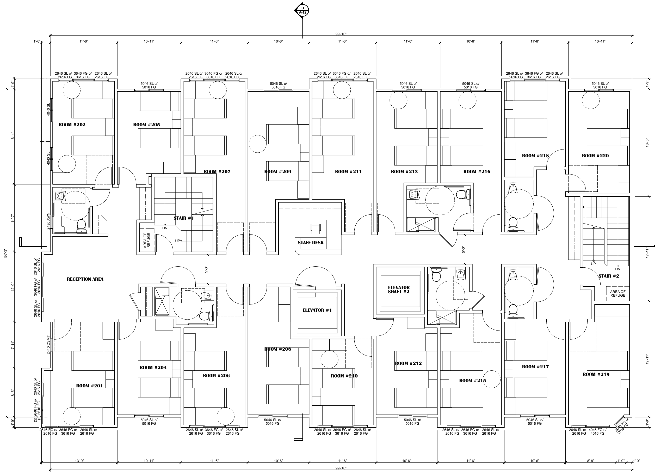
1ST FLOOR PLAN - RCFE (I-1) (Type V Construction) ALL DIM. ARE MEASURED FROM FIN. TO FIN. U.O.N. 1/4" = 1'-0" Bedroom Count Occupants (2 persons/ W/C & Lavatory Count Shower Count
