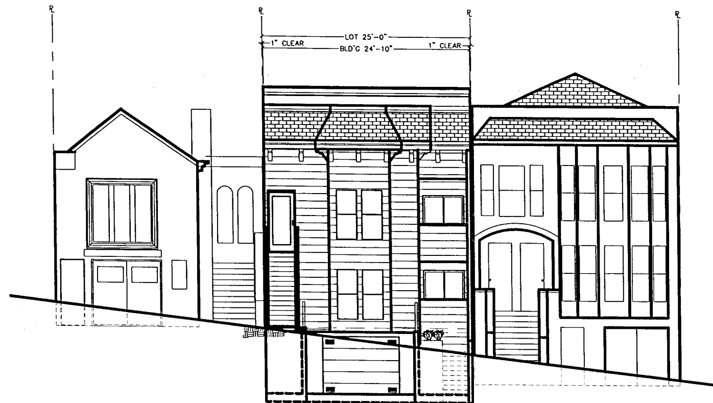
PROPOSED FRONT ELEVATION WITH ADJACENT BUILDING ( 3/16" = 1'-0" )
