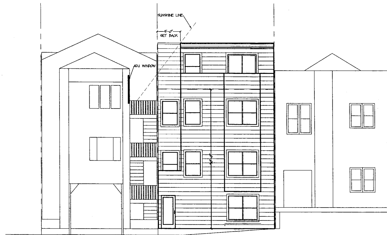
PROPOSED REAR ELEVATION WITH ADJACENT BUILDING ( 3/16" = 1'-0" )
