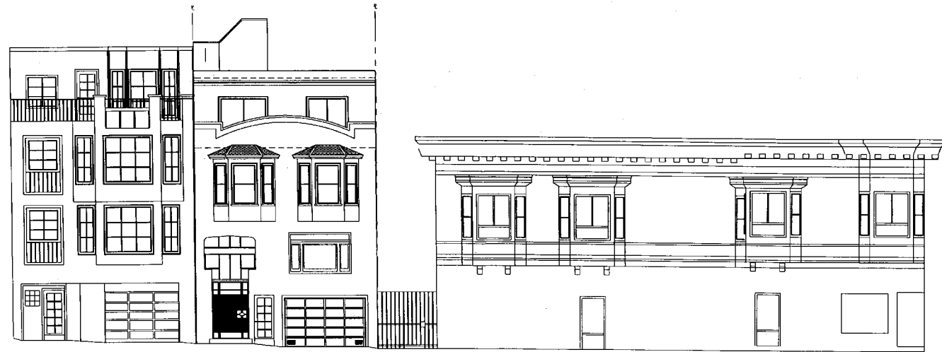
PROPOSED FRONT ELEVATION WITH ADJACENT BUILDING ( 3/16" = 1'-0" )
