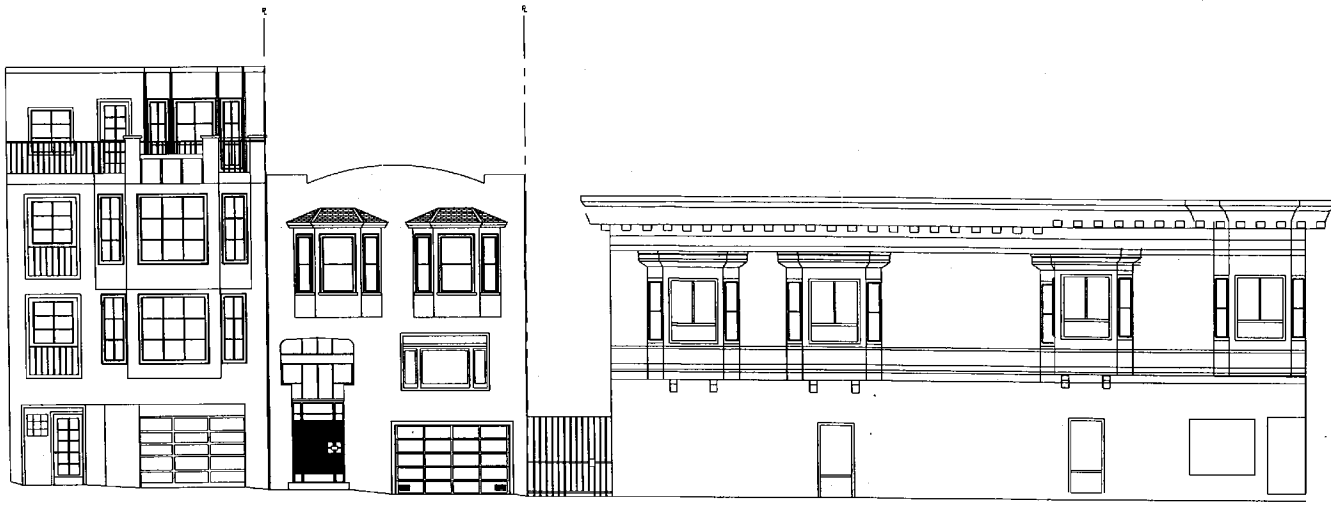
EXISTING FRONT ELEVATION WITH ADJACENT BUILDING ( 3/16" = 1'-0" )
