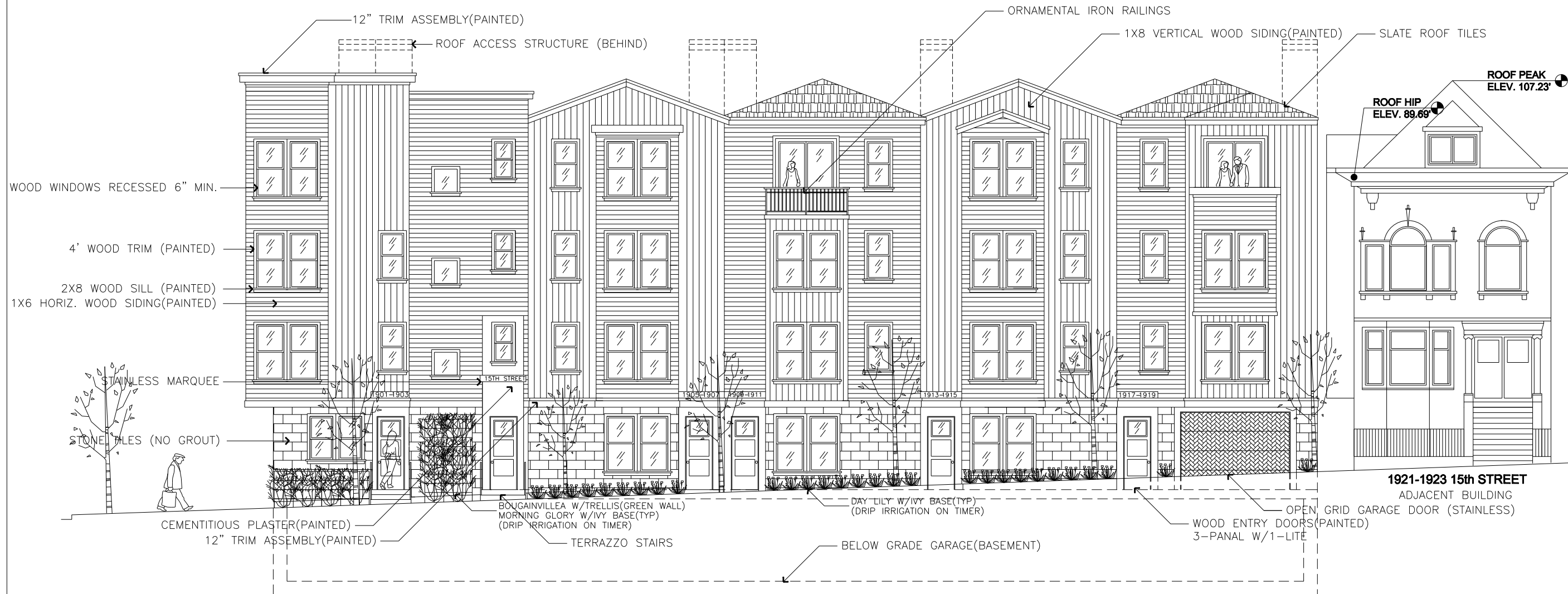
NORTH ELEVATION NOTE: ALL FINISHES ARE THE SAME AT ALL ELEVATIONS UNLESS OTHERWISE INDICATED.
