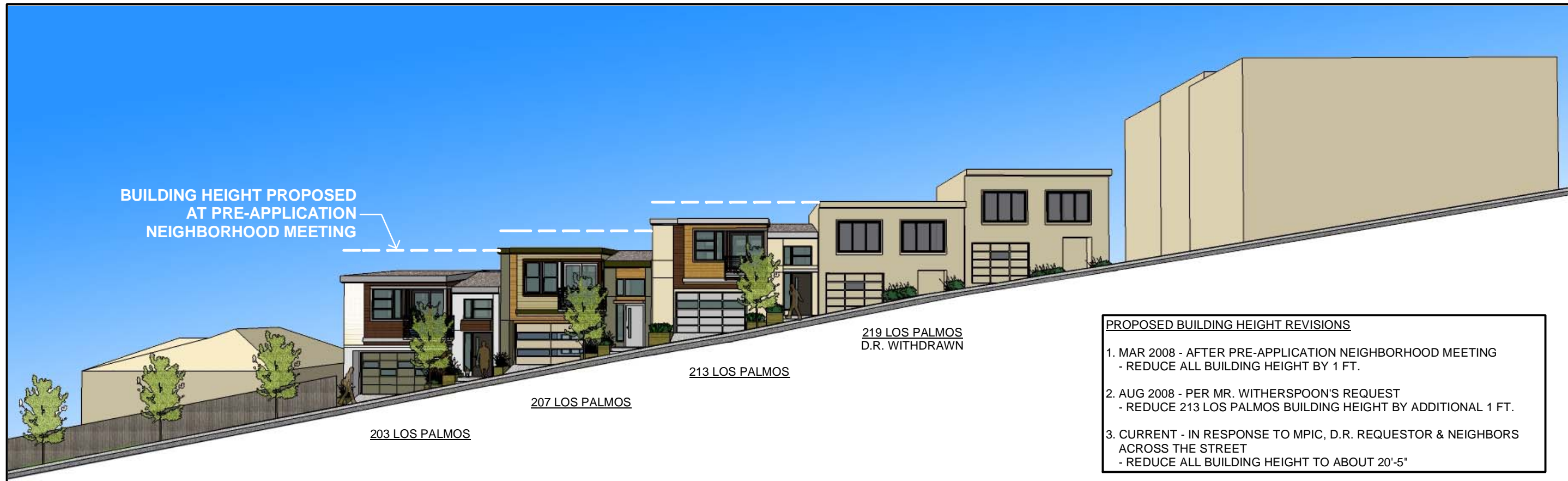
STREETSCAPE SHOWING THE CURRENT PROPOSAL FOLLOWING THE TOPOGRAPHY AND STEP DOWN IN HARMONY WITH THE SLOPE
