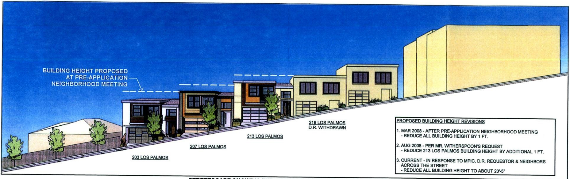
STREETSCAPE SHOWING THE CURRENT PROPOSAL FOLLOWING THE TOPOGRAPHY AND STEP DOWN IN HARMONY WITH THE SLOPE
