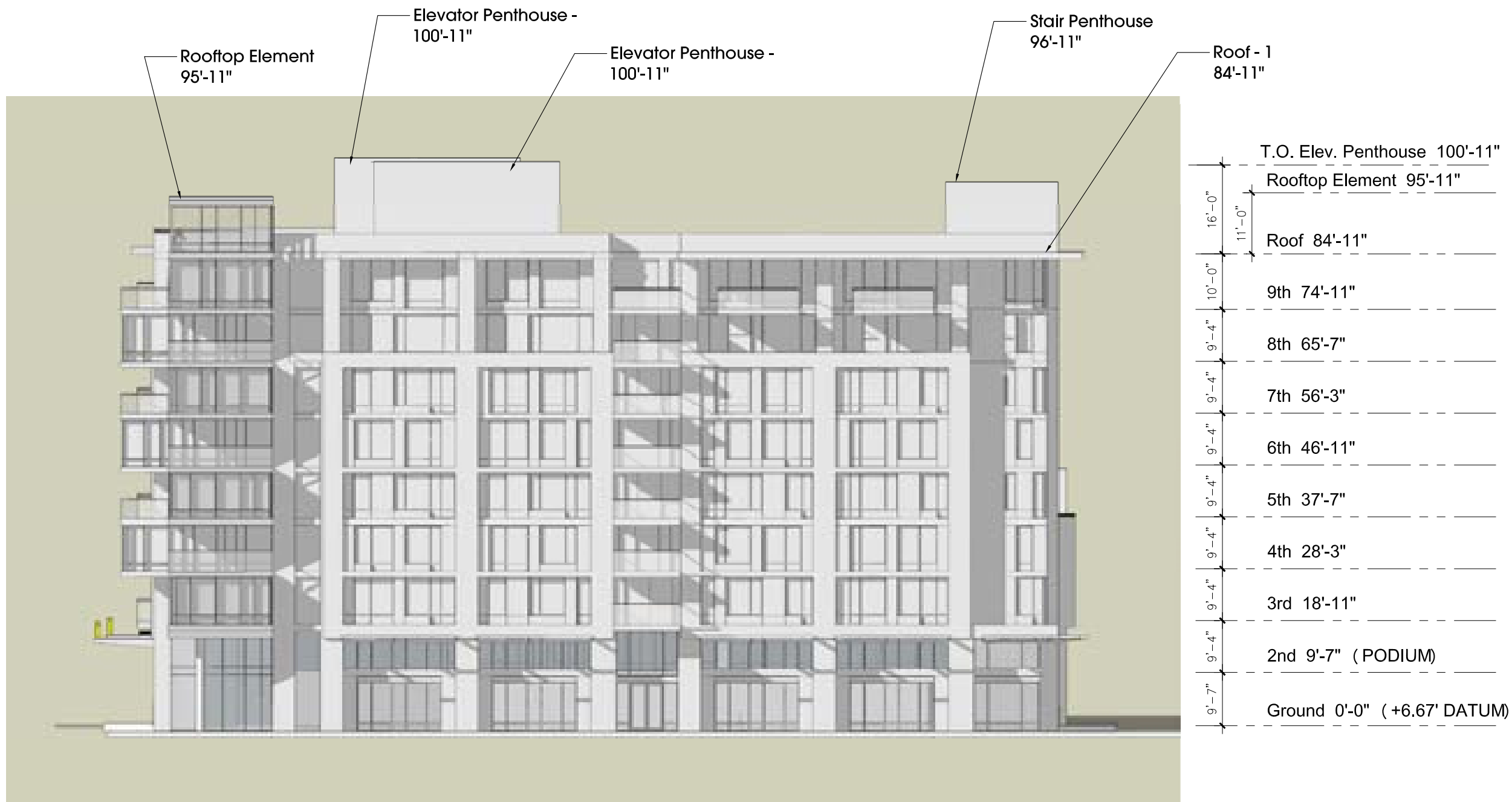
1 FIFTH STREET ELEVATION SCALE: NTS SEE SECTION A3.01 FOR HEIGHT AND DIMENSIONAL INFORMATION
