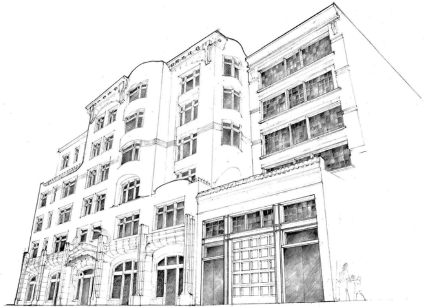
Sketch of proposed project at 1645-1661 Pacific Avenue. Note: Garage entrance at 1661 Pacific Avenue, setback of new construction, and retention of original ornament will preserve the character-defining features of the existing building. Page & Turnbull, April 2008.
