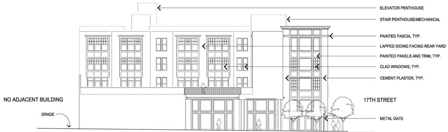
EAST ELEVATION (BLINDWALL - DE HARO STREET BUILDING)
