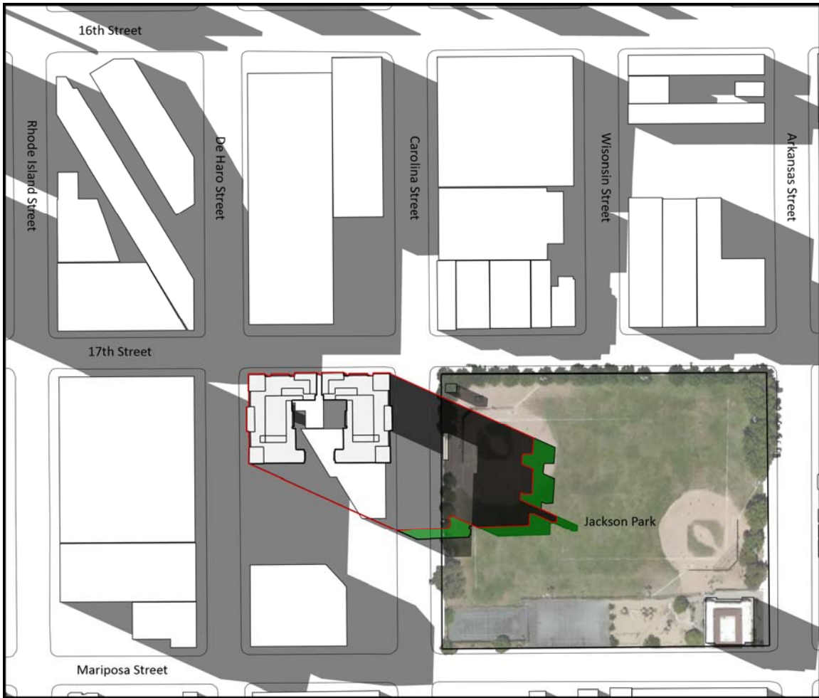
1717 17th Street Shadow Analysis 48' building and 40' building overlay June 21 7:30pm
