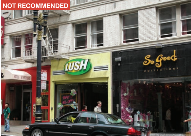
These three storefronts above do not visually relate to one another because of different cladding materials and are discontinuous design from the upper stories to one another.
