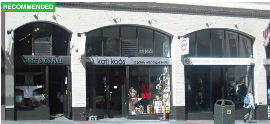
The horizontal features of the three commercial businesses to the left are aligned, relating each storefront to each other and resulting in a cohesive street wall.
