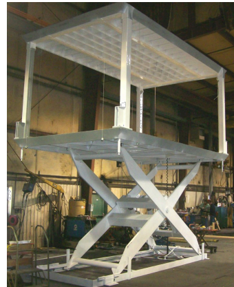
SIMILAR LIFT ASSEMBLY W/ CANOPY
