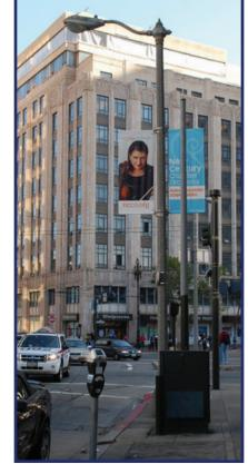
Aggregate concrete streetlight post with pendant arm style cobra luminaire at Larkin St
