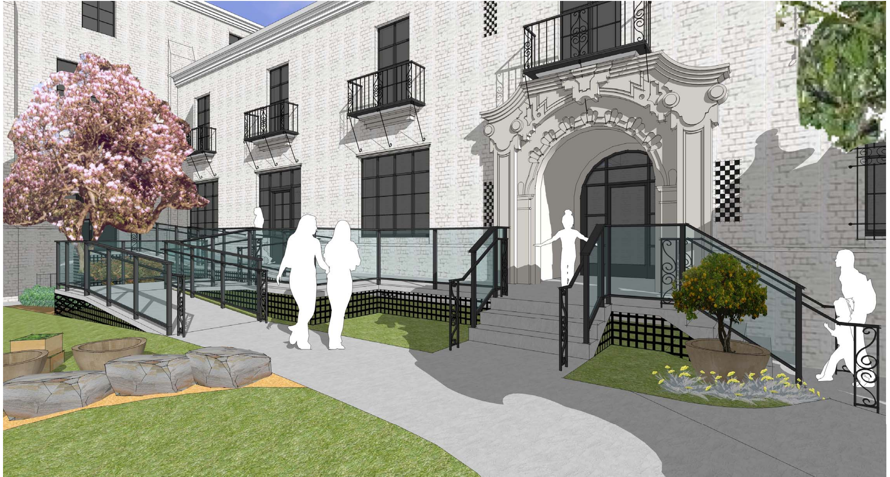
PROPOSED RAMP ELEVATION - STEEL-FRAMED GUARD RAIL WITH GLASS PANELS & DECORATIVE HANDRAIL & PERFORATED BASE SCREEN
