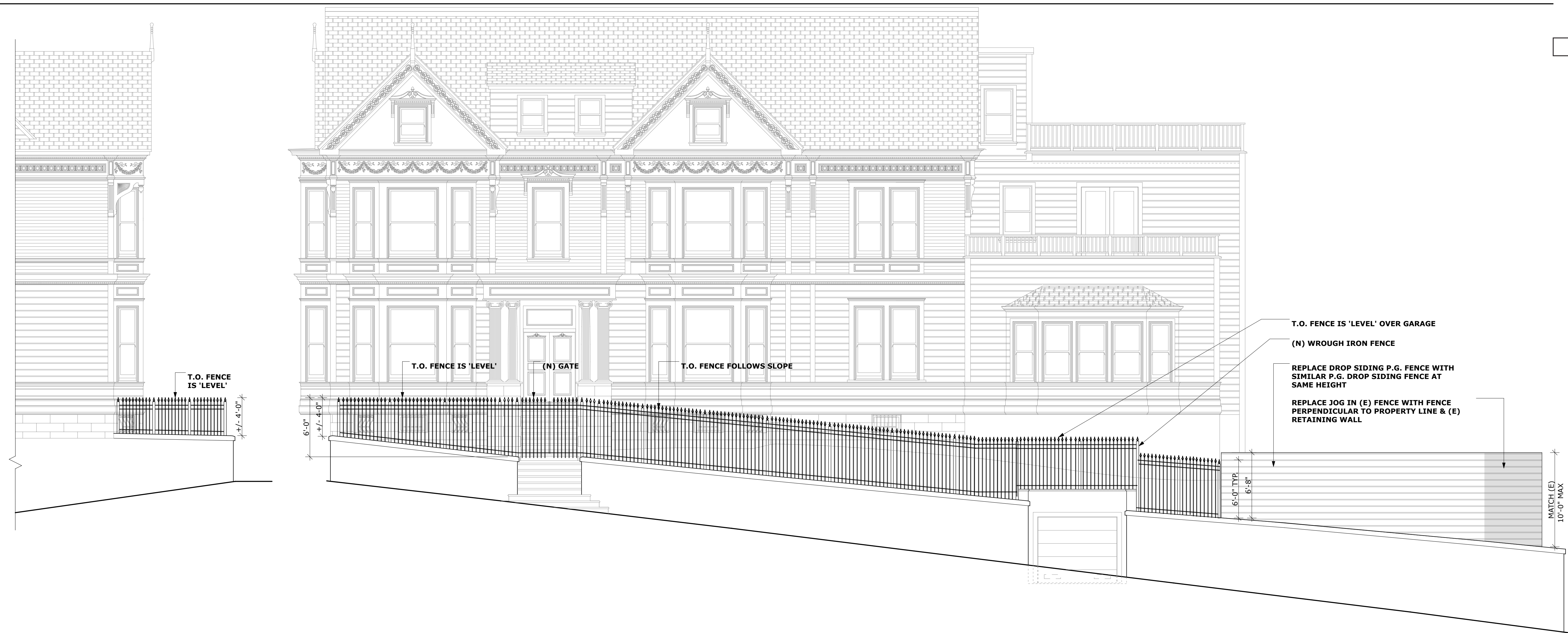
2 ELEVATION: PROPOSED SOUTH & PARTIAL WEST WITH FENCE SCALE: 3/16" = 1'-0"
