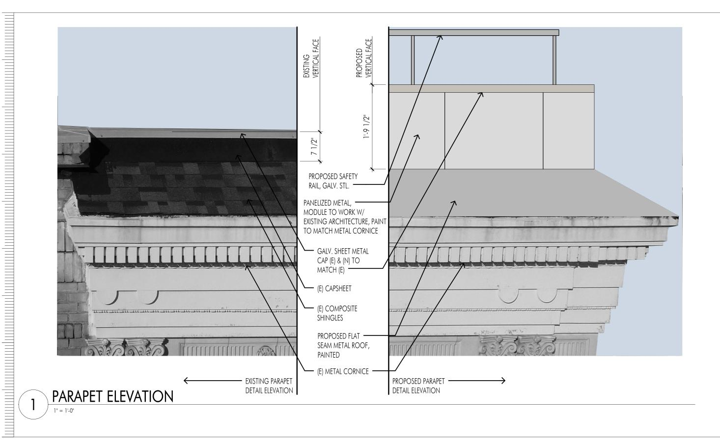
Parapet Elevation Detail
