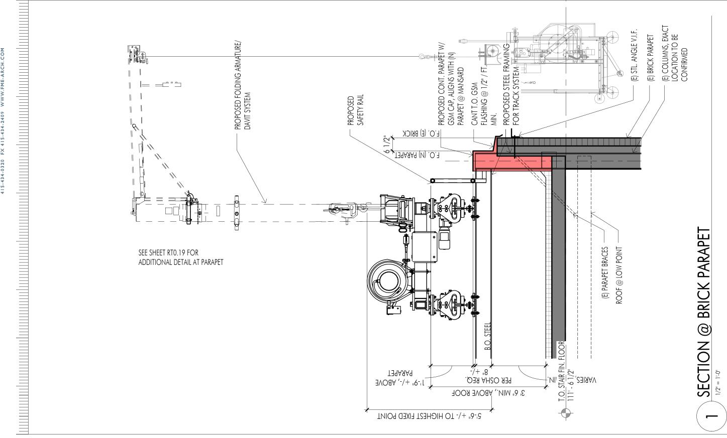
Section @ Brick Parapet
