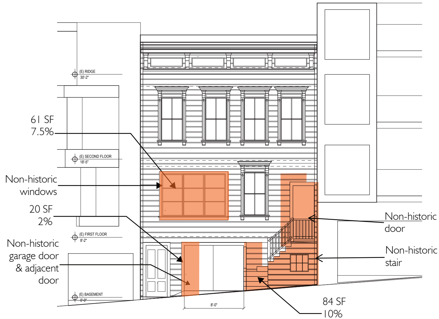
1 EXISTING FRONT ELEVATION
