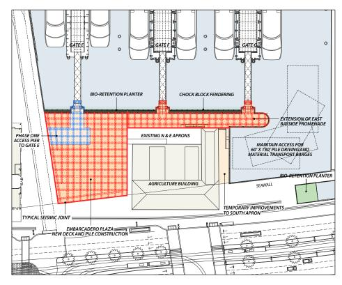
**Figure 30: Preliminary South Basin Structural Concept**
