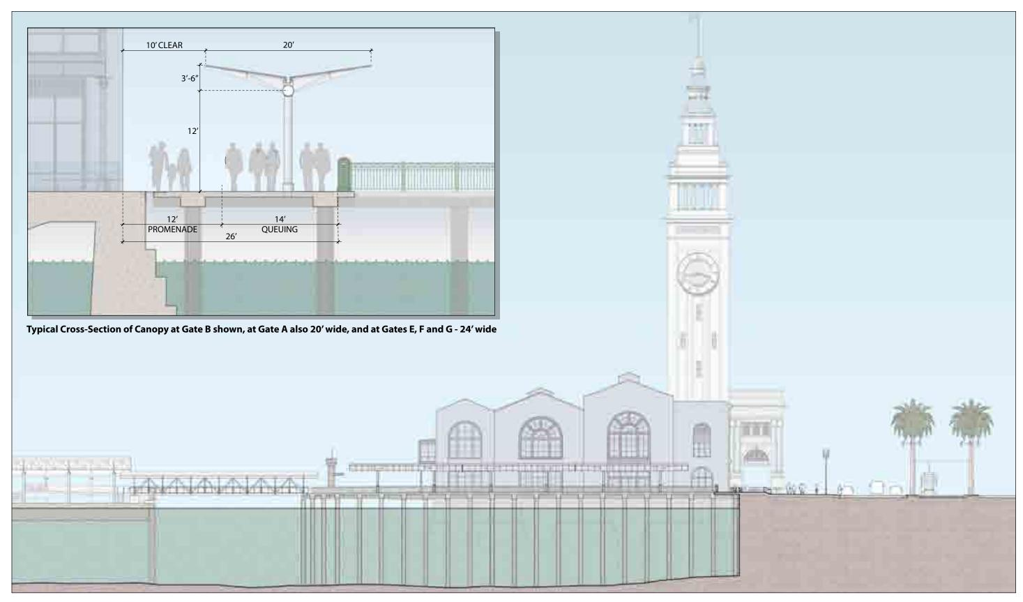
Figure 20: Gate B Queuing Area Canopy Design Concept for Organization, Signage and Weather Protection
