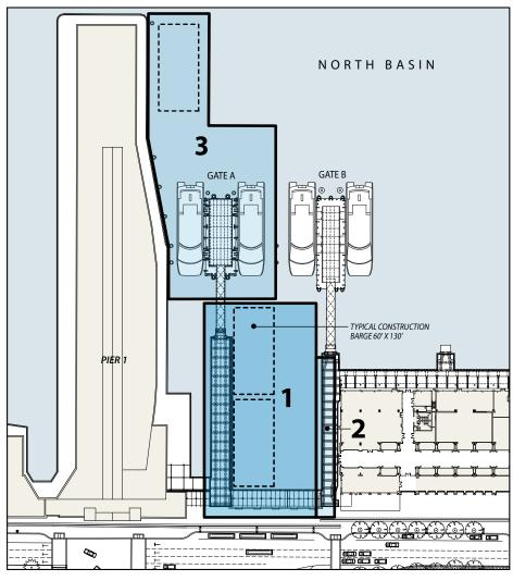
Figure 31: Construction Zones - North Basin
