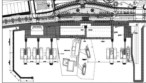
Figure 10: Pier 14 Single Bent Arm Breakwater Option
