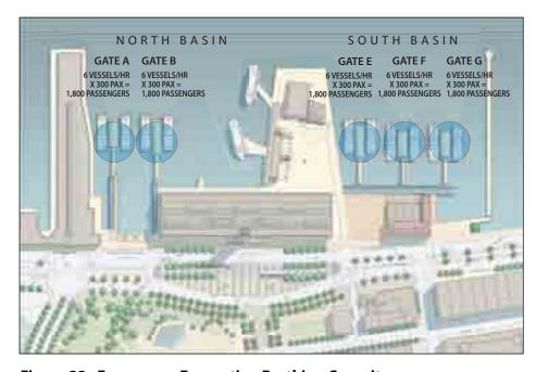
**Figure 23: Emergency Evacuation Berthing Capacity**
