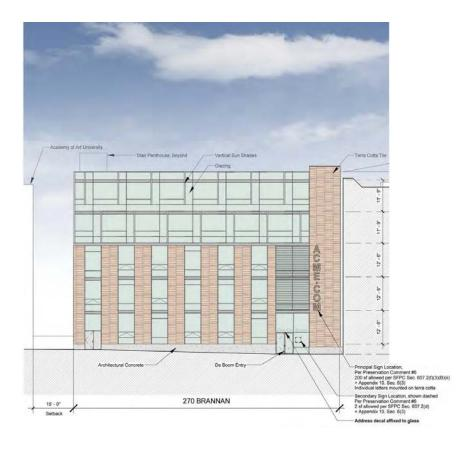
Figure 12: De Boom Street Elevation
