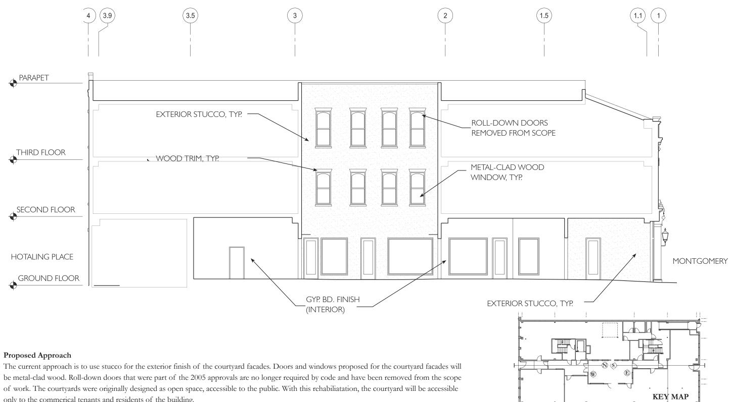
be metal-clad wood. Roll-down doors that were part of the 2005 approvals are no longer required by code and have been removed from the scope of work. The courtyards were originally designed as open space, accessible to the public. With this rehabiliatation, the courtyard will be accessible only to the commerical tenants and residents of the building.
