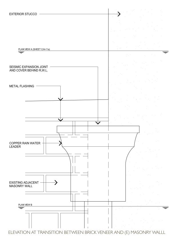
ALIGN FACE OF EXTERIOR STUCCO WITH FACE OF (E)MASONRY WALL **HOTALING PLACE** COPPER RAIN WATER LEADER EXISTING ADJACENT BUILDING SEISMIC EXPANSION JOINT AND COVER WALL FRAMING 2 HR. RATED INSULATED METAL PANEL INTERIOR EXISTING ADJACENT, MASONRY WALL **VARIES** PLAN VIEW OF TRANSITION AT BRICK VENEER TO (E) MASONRY WALL 6"
