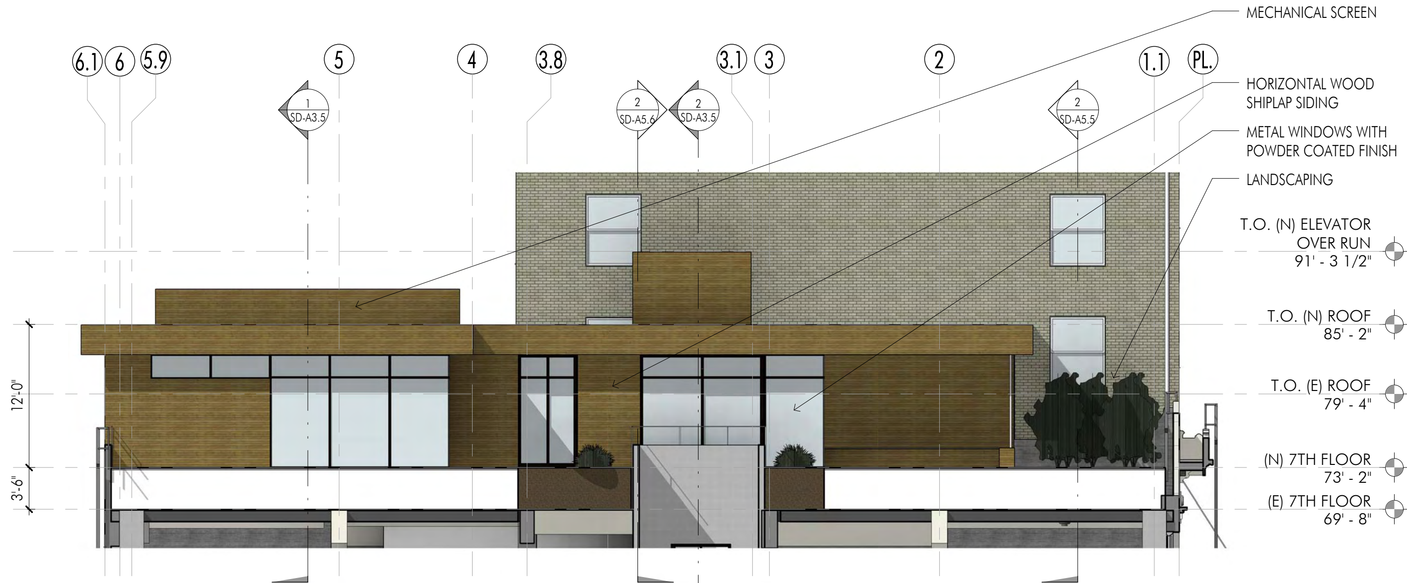
1 ENLARGED EAST ELEVATION - 7TH FLOOR 1/8" = 1'-0"
