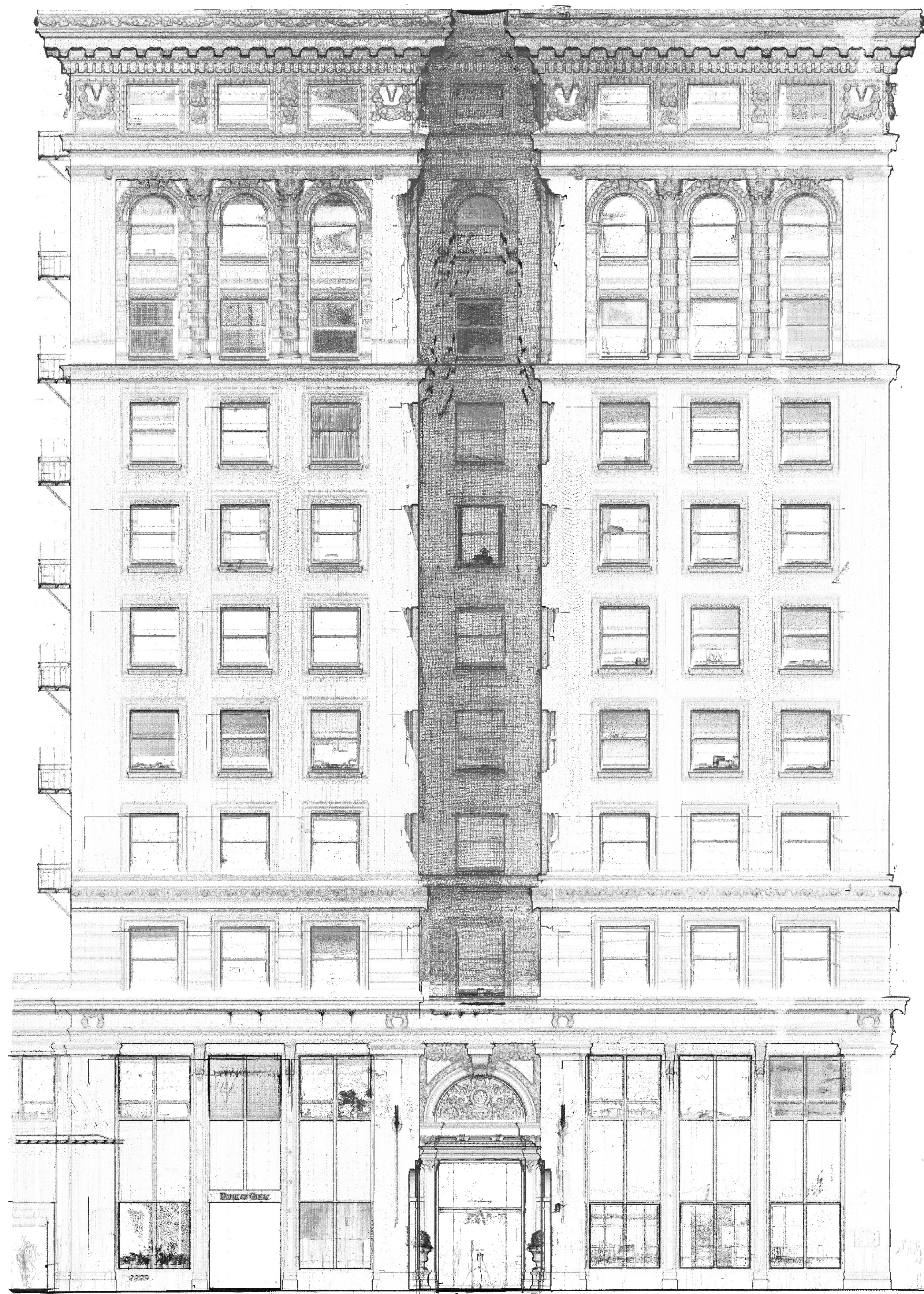
2 ORTHOGRAPHIC PROJECTION OF LASER SCAN DATA - MONTGOMERY STREET FACADE Scale: 1/8" = 1'-0"
