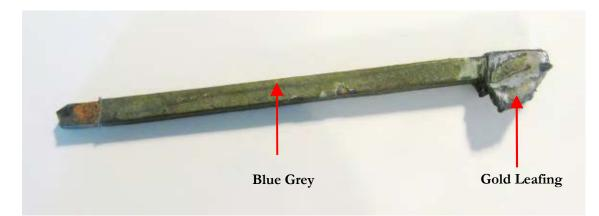
Figure 7: Sample 4, railing spindle.
