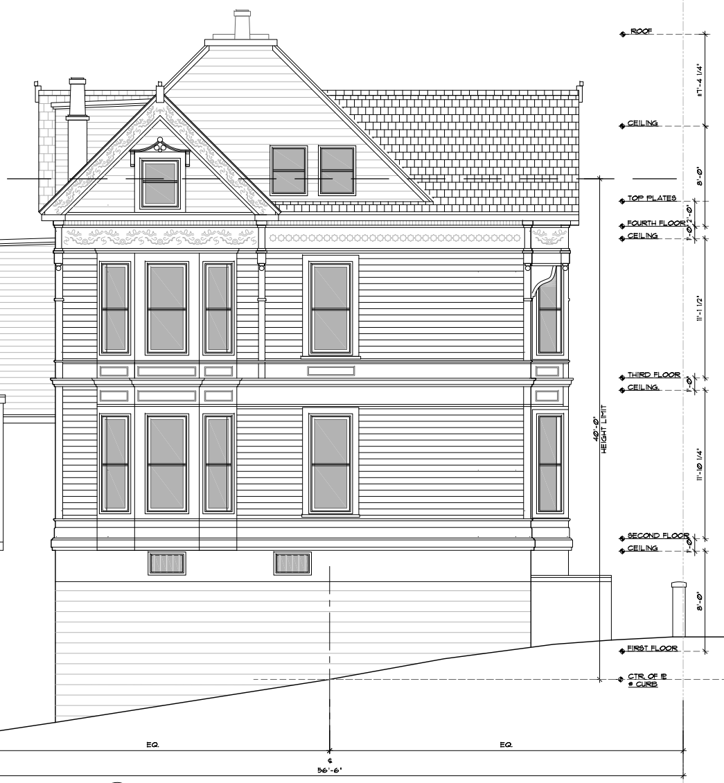
2 EXISTING WEST ELEVATION 1/4" = 1'-0"
