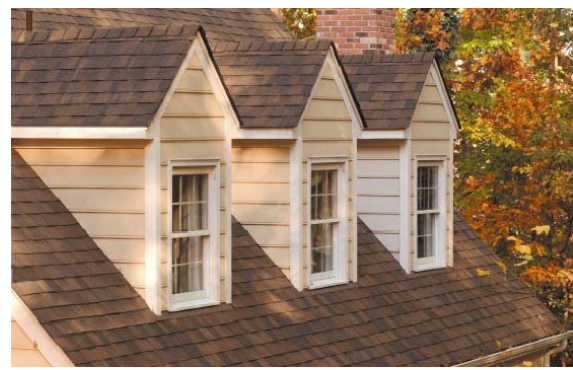
ASPHALT COMPOSITION ROOFING
