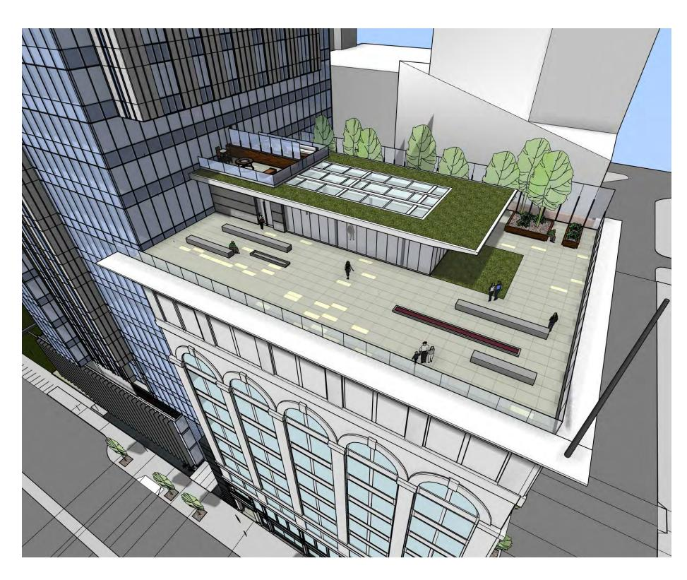
The Aronson Building roof will be rehabilitated to function as a residential amenity outdoor terrace/roof garden for the adjacent new tower. The existing roofing material will be removed and the roof structure will be selectively demolished. A new structural roof diaphragm will provide a seismic upgrade and support required for the exterior cornice, parapet anchorage, landscaped roof terrace, and new solarium will be installed.
