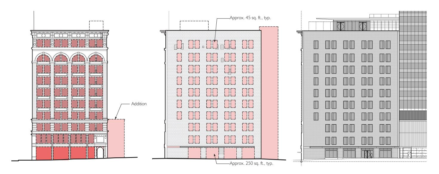
Third Street elevaton (east facade) showing addition at north facade to be removed
