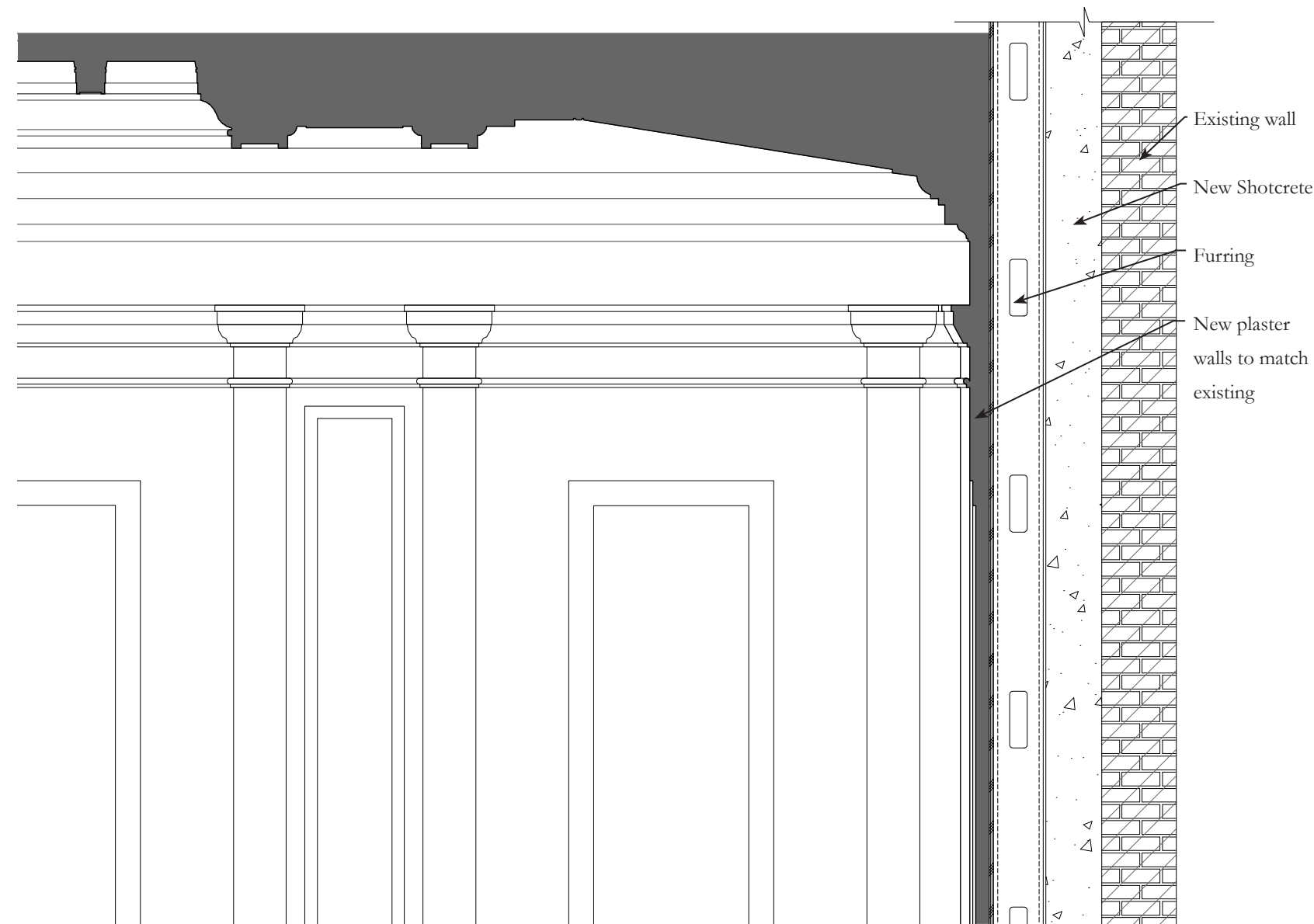
Drawing showing shotcrete reinforcement of walls
