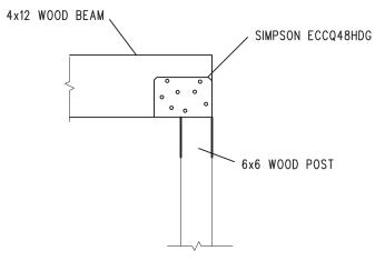
4 POST TO BEAM CONNECTION SCALE: 1" = 1'-0"
